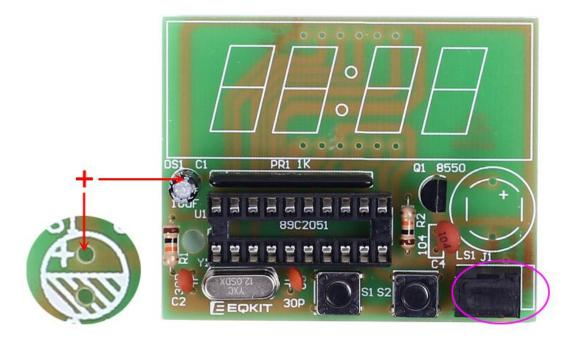
Step 6: Install 1pcs 5V Active Buzzer at LS1 and pay attention to its installation direction. The buzzer and PCB each have a mark '+' that are used to determine the installation direction.
